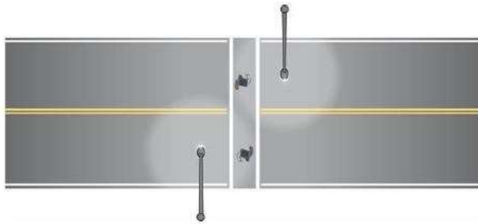
Figure 6.9.3.4: Cross Walk Lighting Pole Placement
